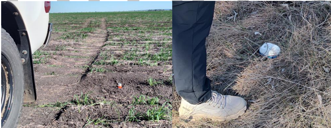
Plate 3-5: Installed Geophone and Accelerometer nodes (Source: M.Kneipp, 2026)
