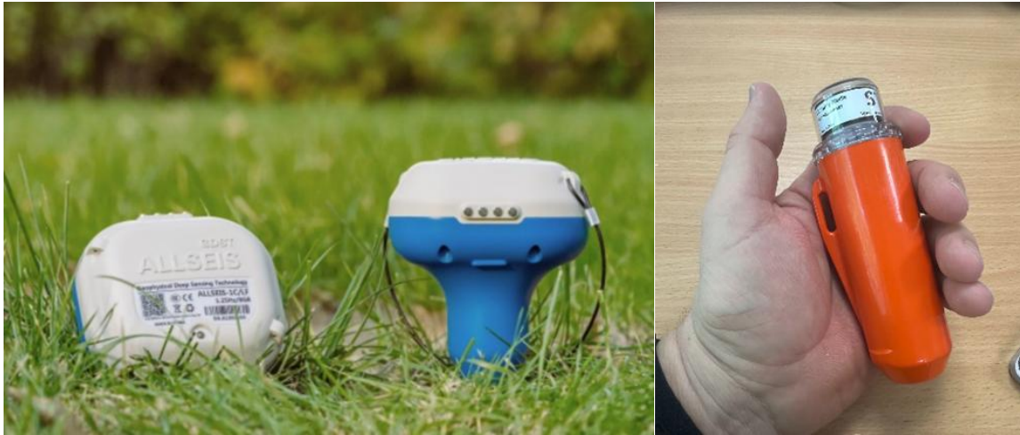
Plate 3-4: Example Geophone and Accelerometer node types (Source: M.Kneipp, 2026)
